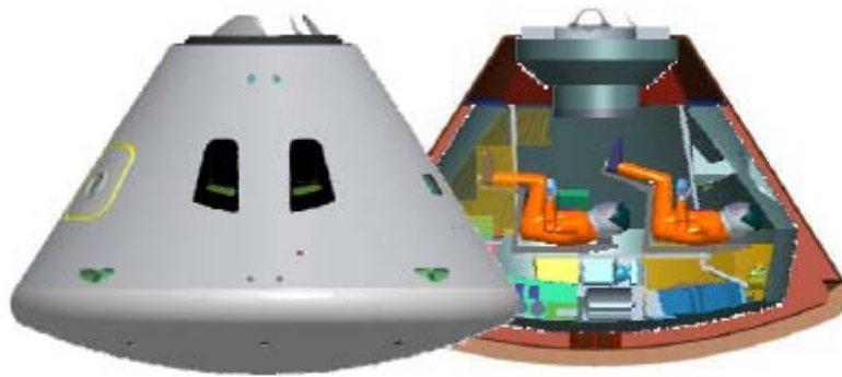
Vertical cross-section of the Orion crew module (NASA Concept)
